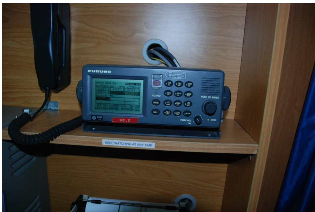
MF/HF Transceiver (SSB)
