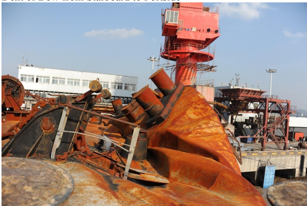
Dent of Bow from Starboard to Portside
