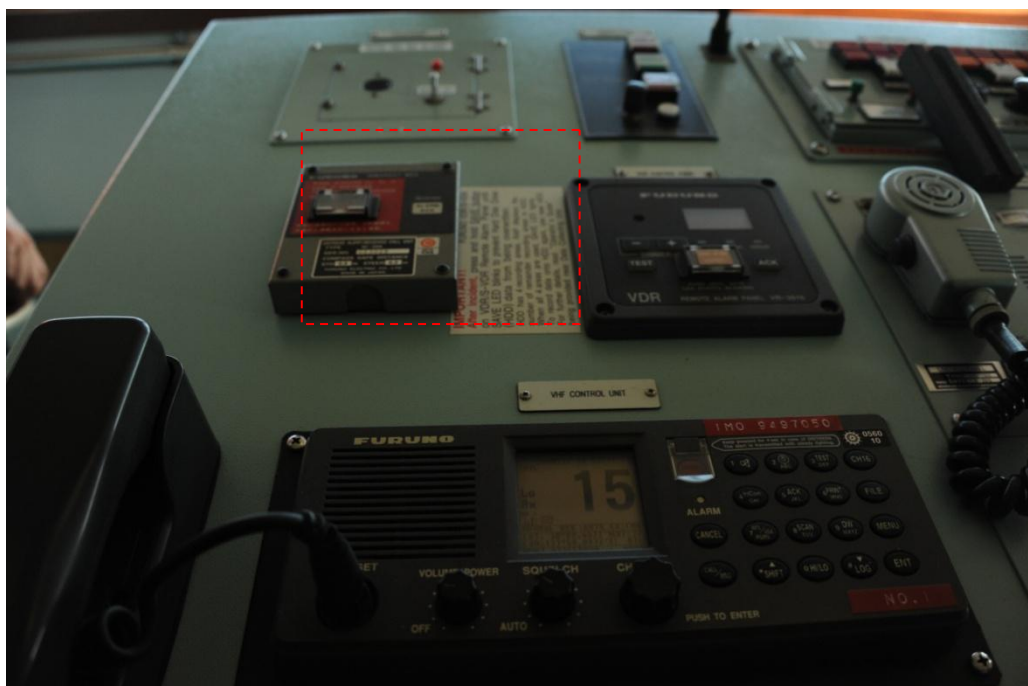
Alarm button of Sat C
