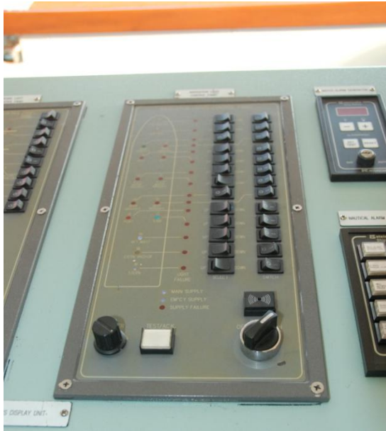
Control panel of Navigational Lights
